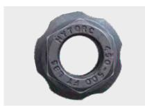
GRIP-TIGHT™ Nuts have M22X1.5 threads, 33mm hex, 27mm height and a 46mm washer diameter. The two-piece GRIP-TIGHT™ Nuts comply with technical requirements of SAE J1965. Cross Reference PN's: 39773, 39874, 39702, M3979, 39691, 39949, 201.3013, 13-3057, E-9020, W-525, R009020, 511034, KB9020,WA075037, 20857204, 1649492C1, E6HZ-1120-A, MF110343, and MF111026.
